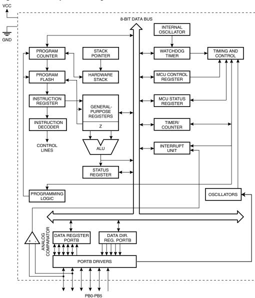
Figure 1. The ATtiny11 Block Diagram
